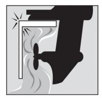
Many trolling plates will fail under the pressure of . accidental acceleration with the plate locked in the down position.
